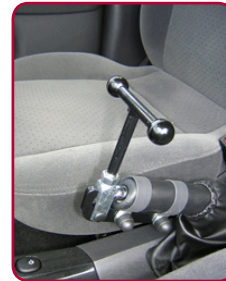
Quick release option allows the Steering Ball to be moved by others driving the car Tripod steering Aid
