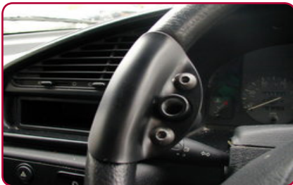
Quick release option allows the Steering Ball to be moved by others driving the car Tripod steering Aid
