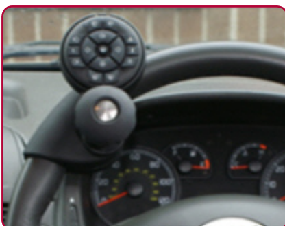
Infrared control unit attached to Steering Wheel Ball. To activate the function you require you simply press the button of that function.
